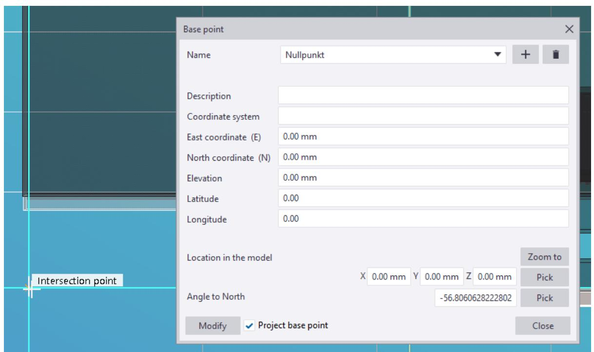
11. Invert the X and Y offsets. Adjust the Z offset if necessary.
