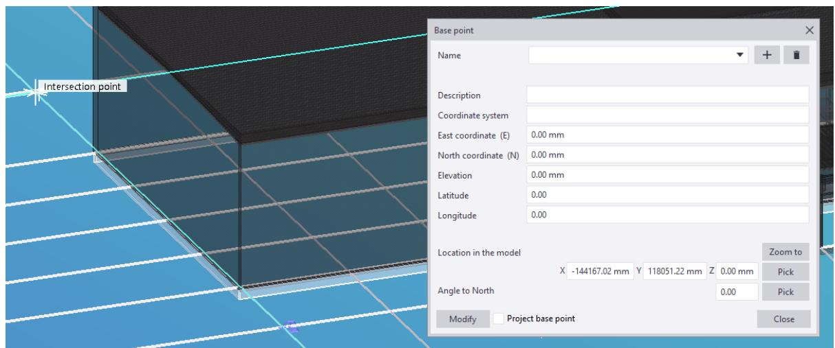
6. Set **X**, **Y** and **Z** offsets to 0 and invert the **Angle to North**.
